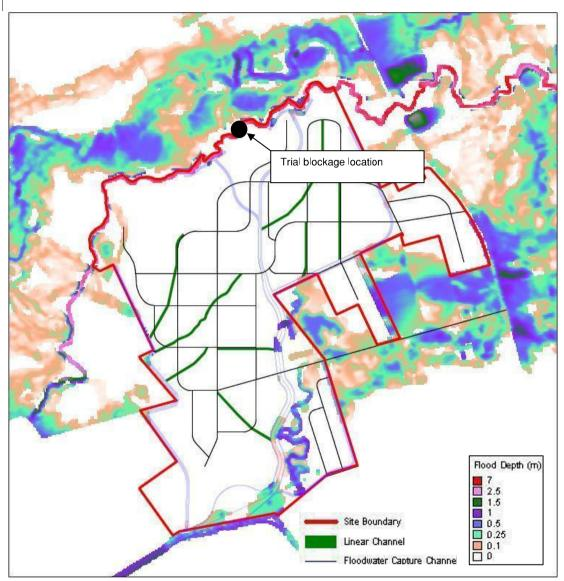
Figure 4.7 - 100 year ARI floodplain with a 25 percent blockage of Gawler River at Location 1
