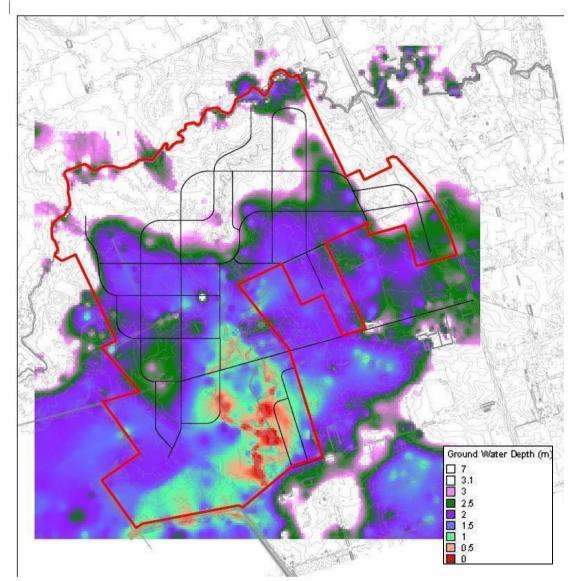
Figure 5.1 - Depth to Groundwater within 3m of existing surface level.
