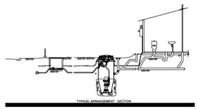
Figure 3.1 Pressure system layout Diagram obtained from Environmental Systems Limited
