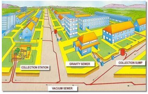
**Fig 3.2 Typical Scheme Layout** Diagram provided by Flovac Pty Ltd
