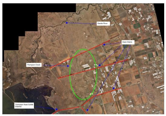
Figure 2.2 – Existing Stormwater Infrastructure
