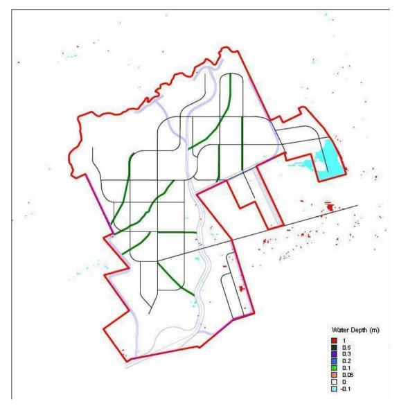
Figure 4.6 - Predicted difference in 100 year ARI Flood elevations with and without the proposed fill to the District Centre and Mixed Use precinct.
