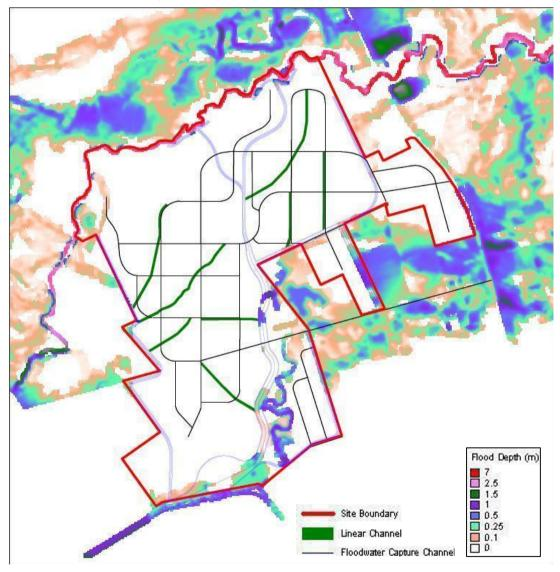
Figure 4.5 - 100 year ARI event in Gawler River with proposed Flood Protection Channels and fill in a section of the Proposed District Centre and Mixed Use precinct.
