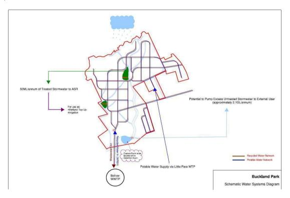
Figure 6.1 Buckland Park Water and Recycled Water Supply Schematic
