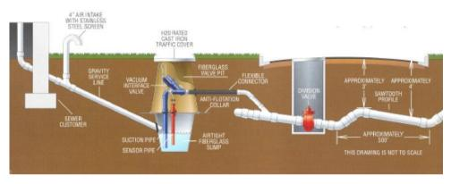
Figure 3.3 Saw-tooth Design
