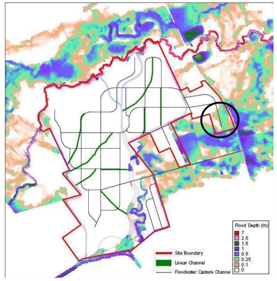
Figure 4.4 - 100 year ARI event in Gawler River with proposed Flood Protection Channels
