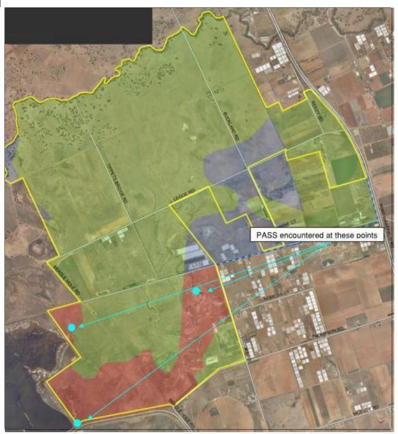
Figure 5.3 - Potential acid sulphate soil locations
