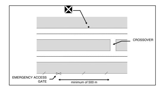
Figure 2: Preferred stagger of access gate and crossover
