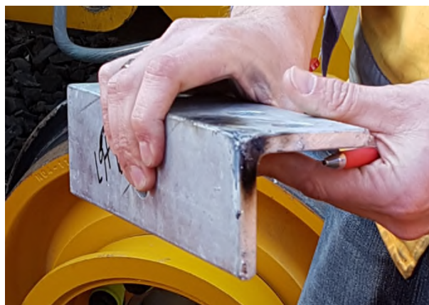
The bracket showing the burn marks from the electrical arcing
