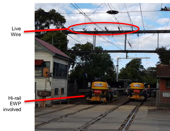
The Kooyong Station level crossing, overhead structure and Hi-rail EWP involved in the incident
