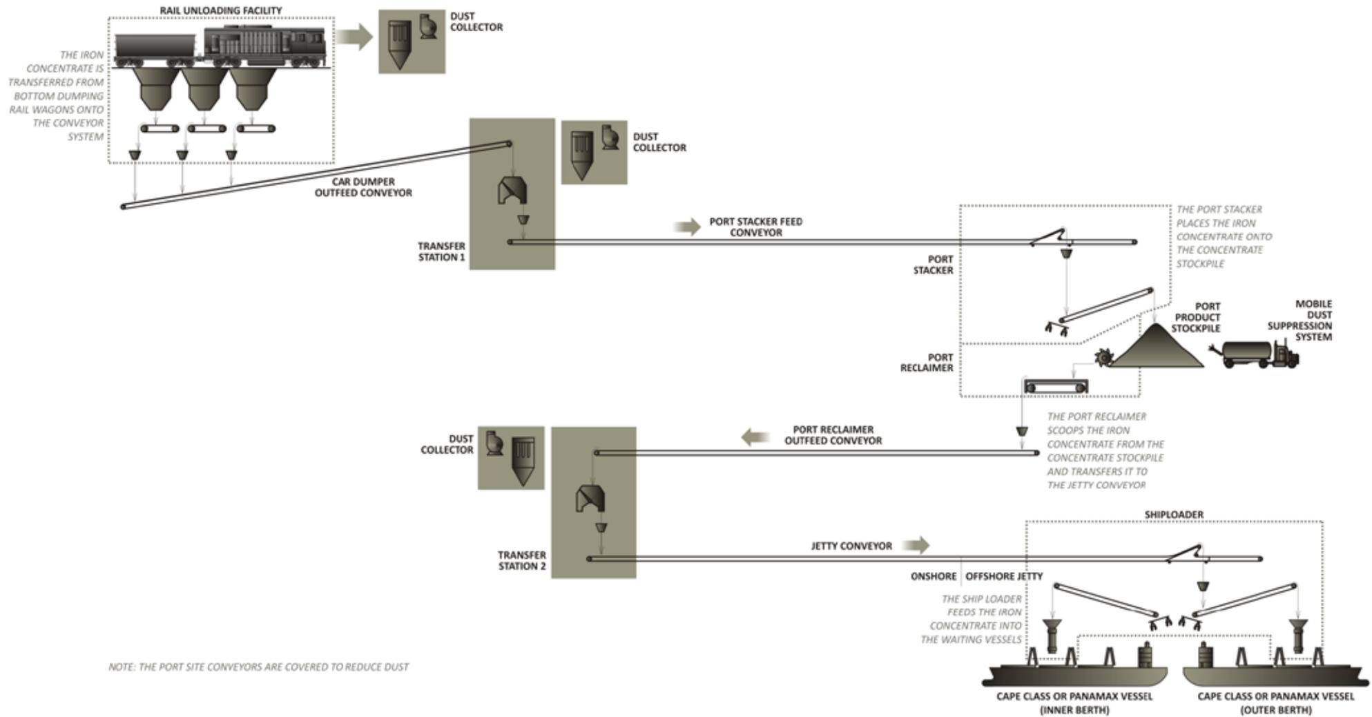
Figure 10-3 Port Site Simplified Process Flow Diagram Showing Materials Handling
