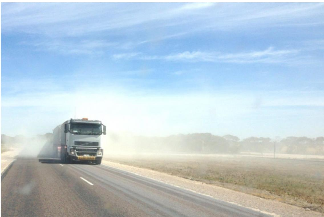
Plate 10-3 Truck-Generated Dust on Sealed Road
