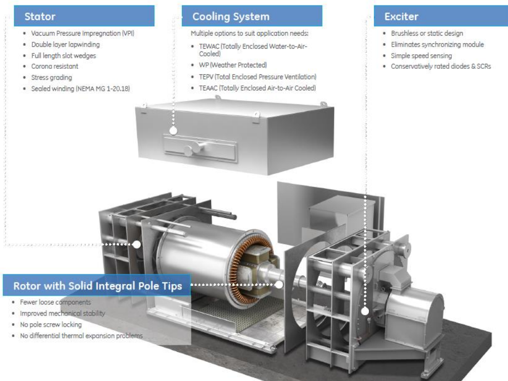
Figure 4-5 Synchronous Condenser Main Components (source: gegridsolutions.com)
