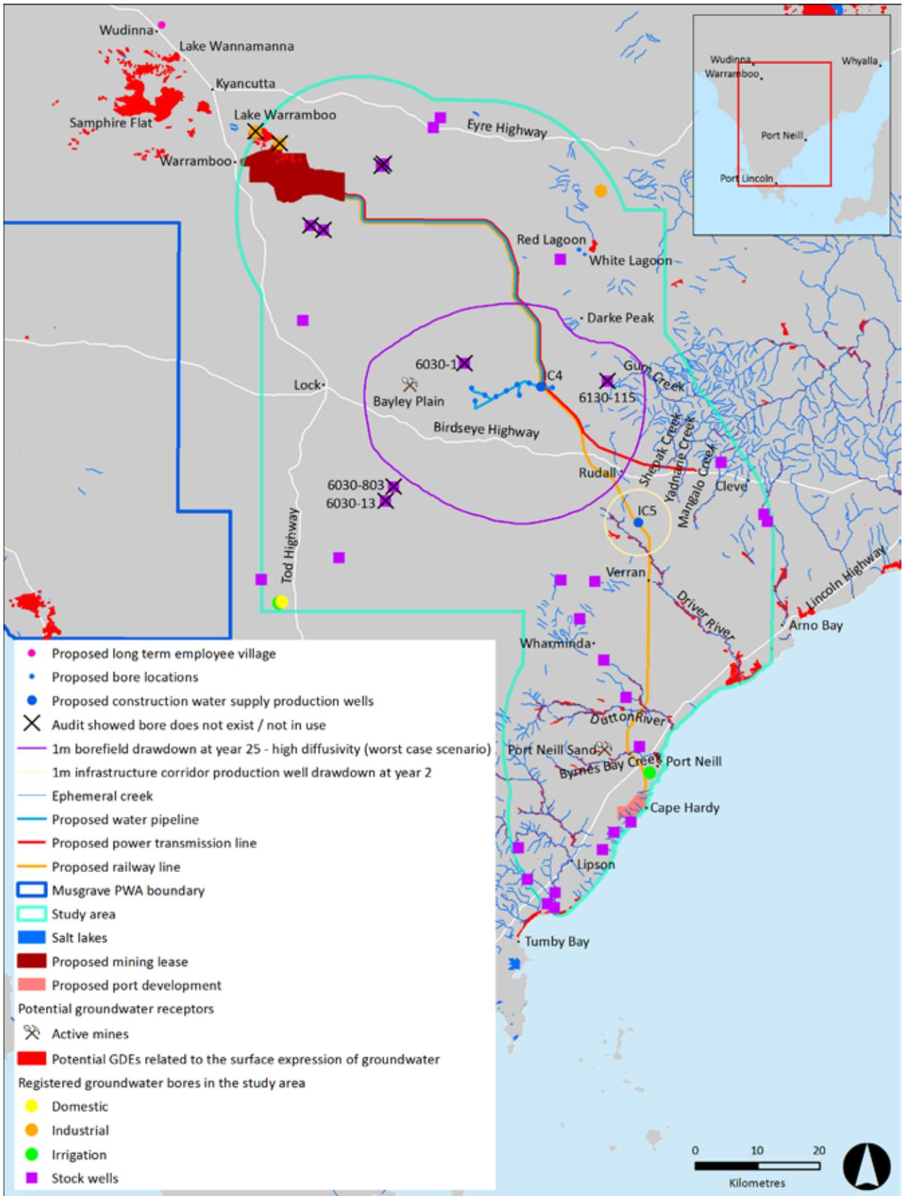
Figure 16-6 Predicted Zone of Drawdown Influence (Worst Case Scenario) and Receptor Identification
