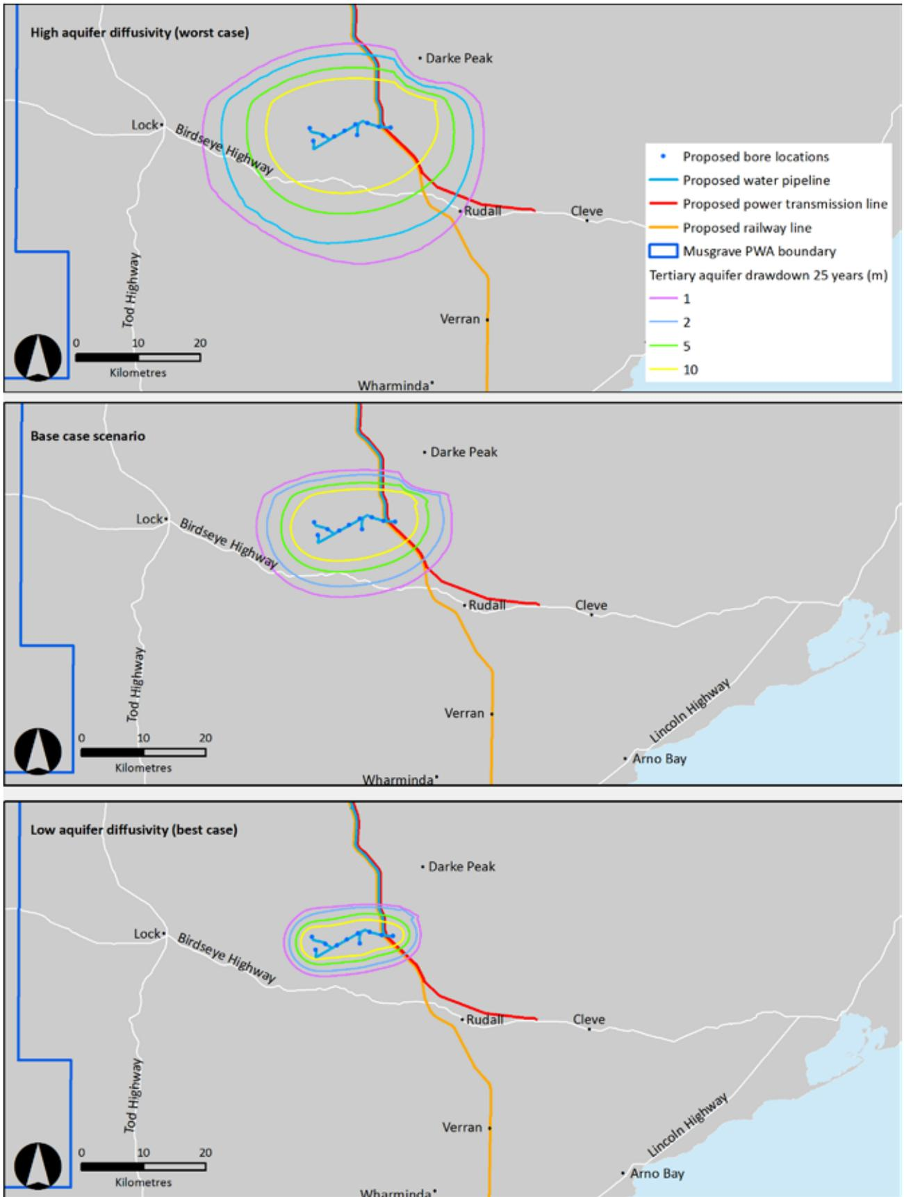
Figure 16-5 Predicted Drawdown Following 25 Years of Proposed Borefield Operation
