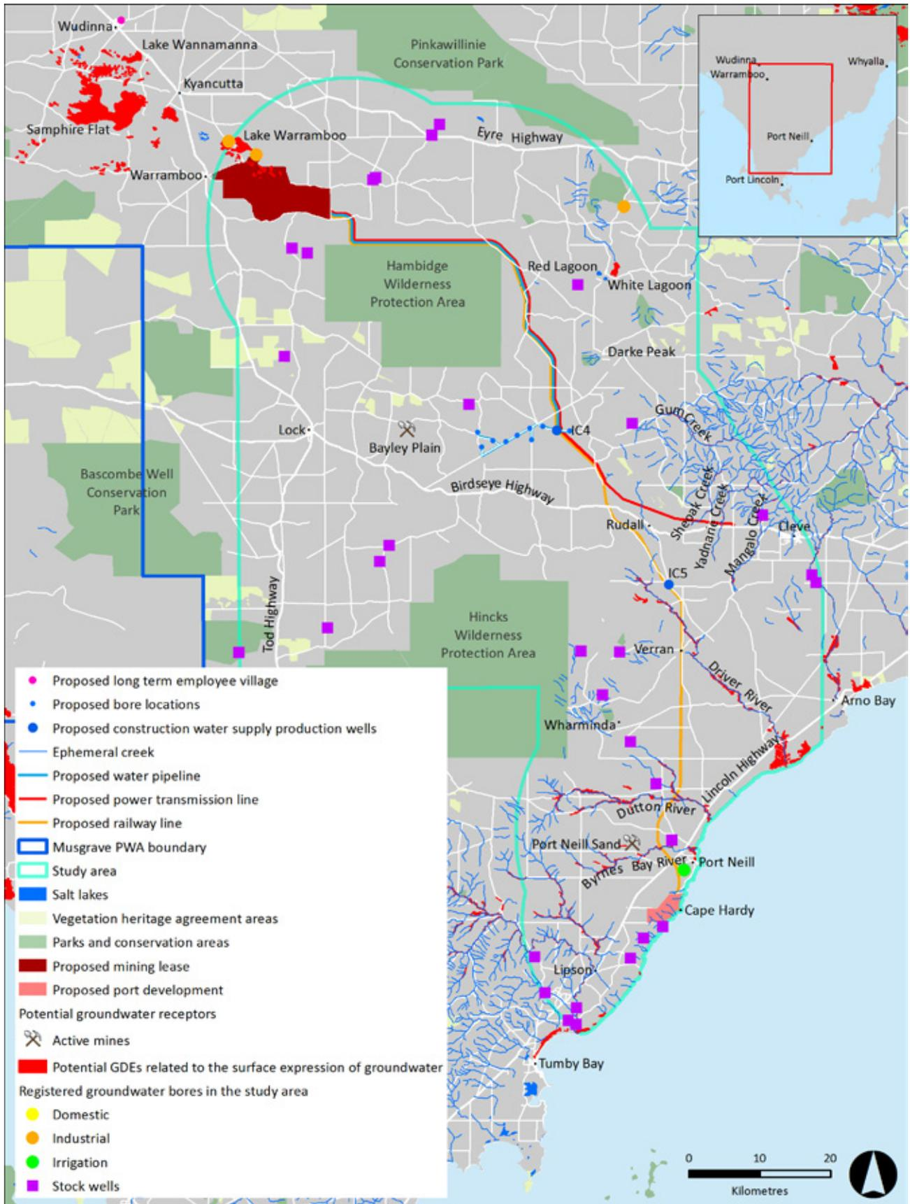
Figure 16-3 Potential Groundwater Receptors in the Study Area
