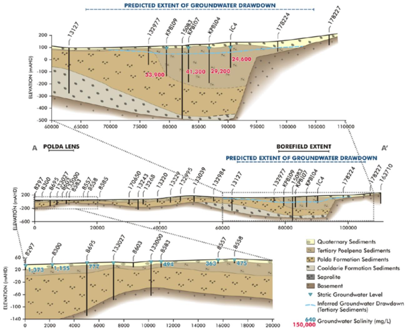
Figure 16-2 Hydrogeological Cross Section – Proposed Borefield to Musgrave PWA
