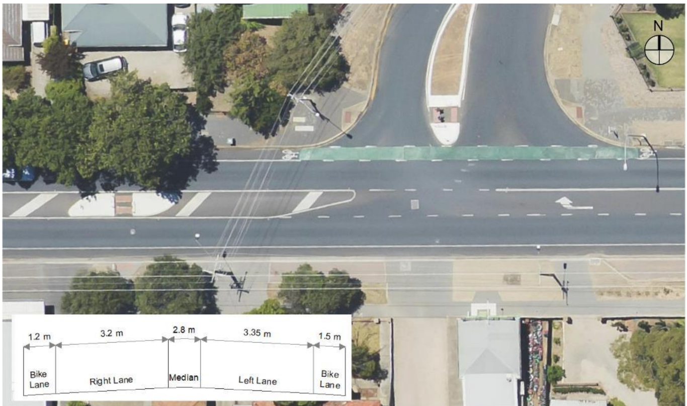
Figure 4: Springbank Road Midblock Cross-section (refuge and bike lane widths vary – refer Appendix A)
