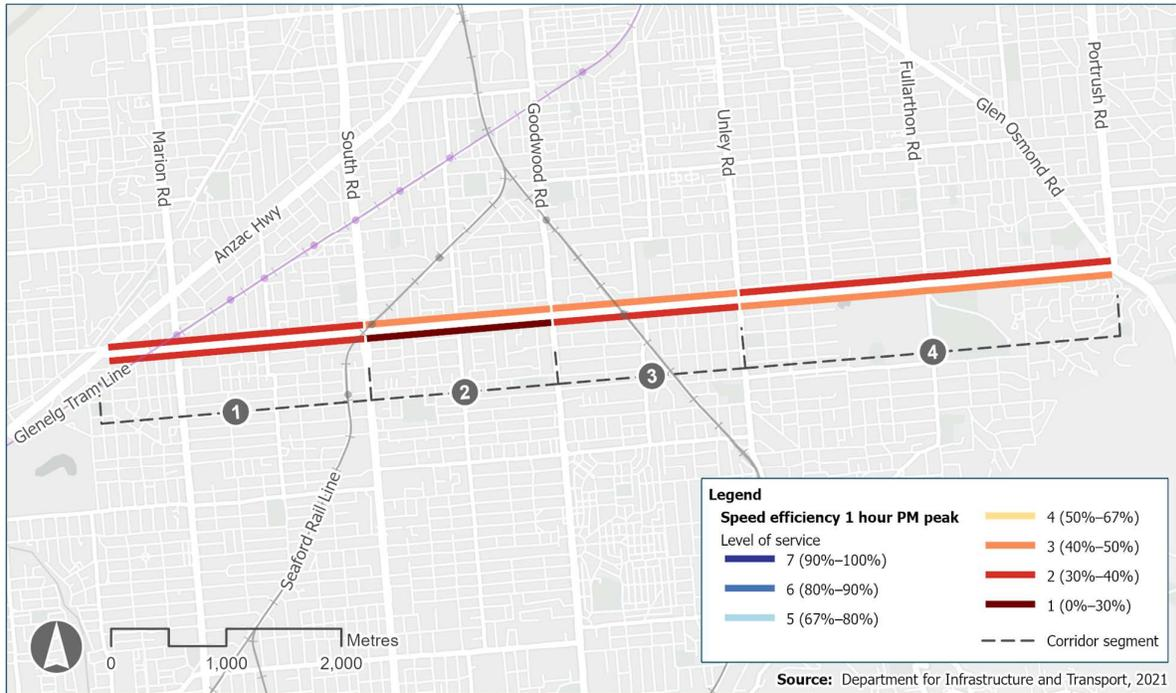
Figure 58: Average speed efficiency along corridor for 1-hour PM peak
