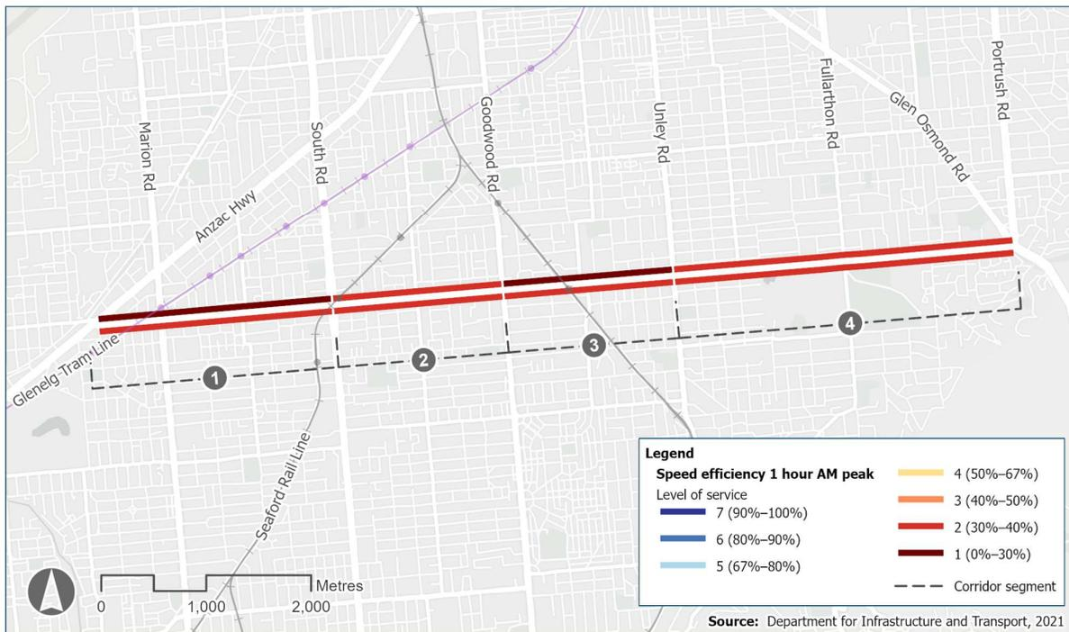
Figure 57: Average speed efficiency along corridor for 1-hour AM peak
