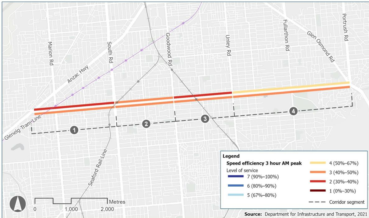
Figure 59: Average speed efficiency for 3-hour AM peak period
