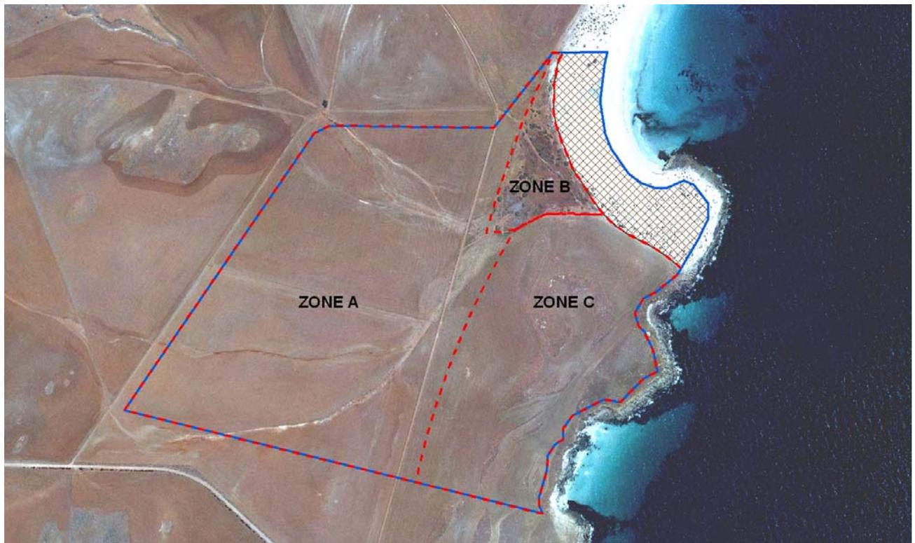
The boundaries between the zones cannot be interpreted accurately on the basis of the relatively few widely spaced test pits and boreholes placed during the investigation and hence the interzone boundaries shown on the Figure 3A must be regarded as approximate only.
