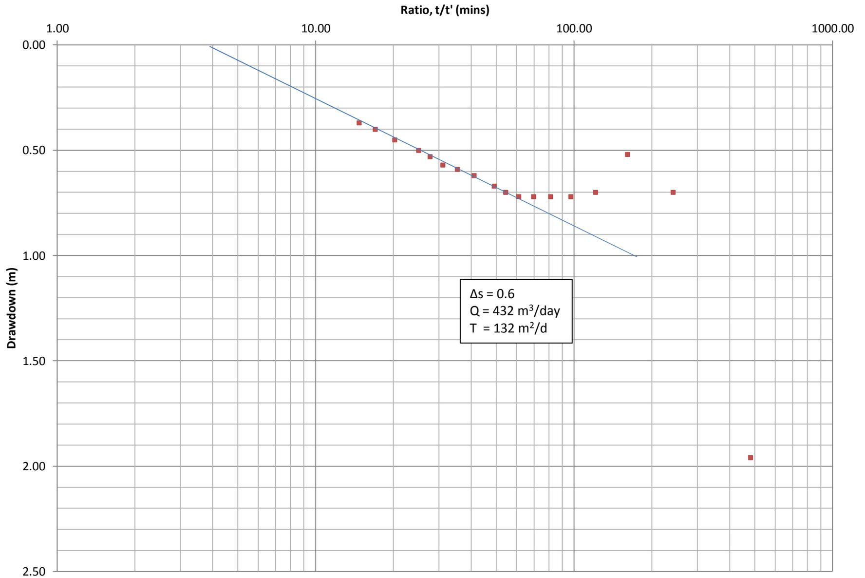
Iron Road CEIP Constant Rate Test and Recovery Data
