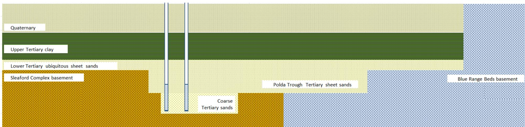
**Figure 4-1: Hydrogeological Model Conceptualisation (North – South Section)**
