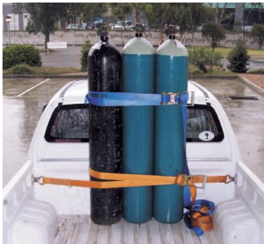
Example of correct positioning and restraining of gas cylinders.
