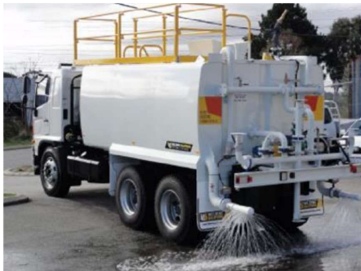
Water carts will be used to mitigate dust.
