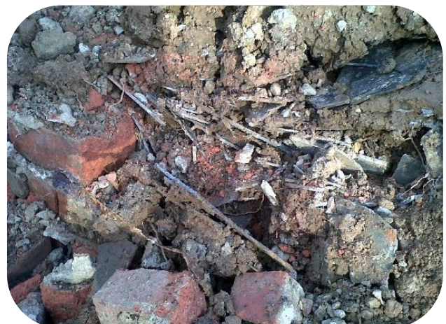
Asbestos containing material (ACM) mixed through dumped construction demolition waste
