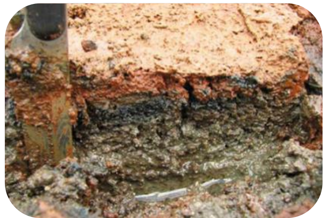
ASS will clod together to create a plate effect. It is water logged with a rotten odour
