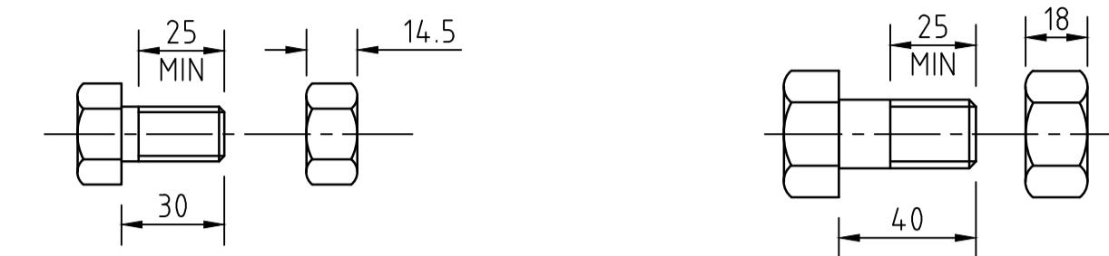
M16x30 BOLT (FB02) & NUT (FN01) BLOCKOUT CONNECTION TO C-POSTS
