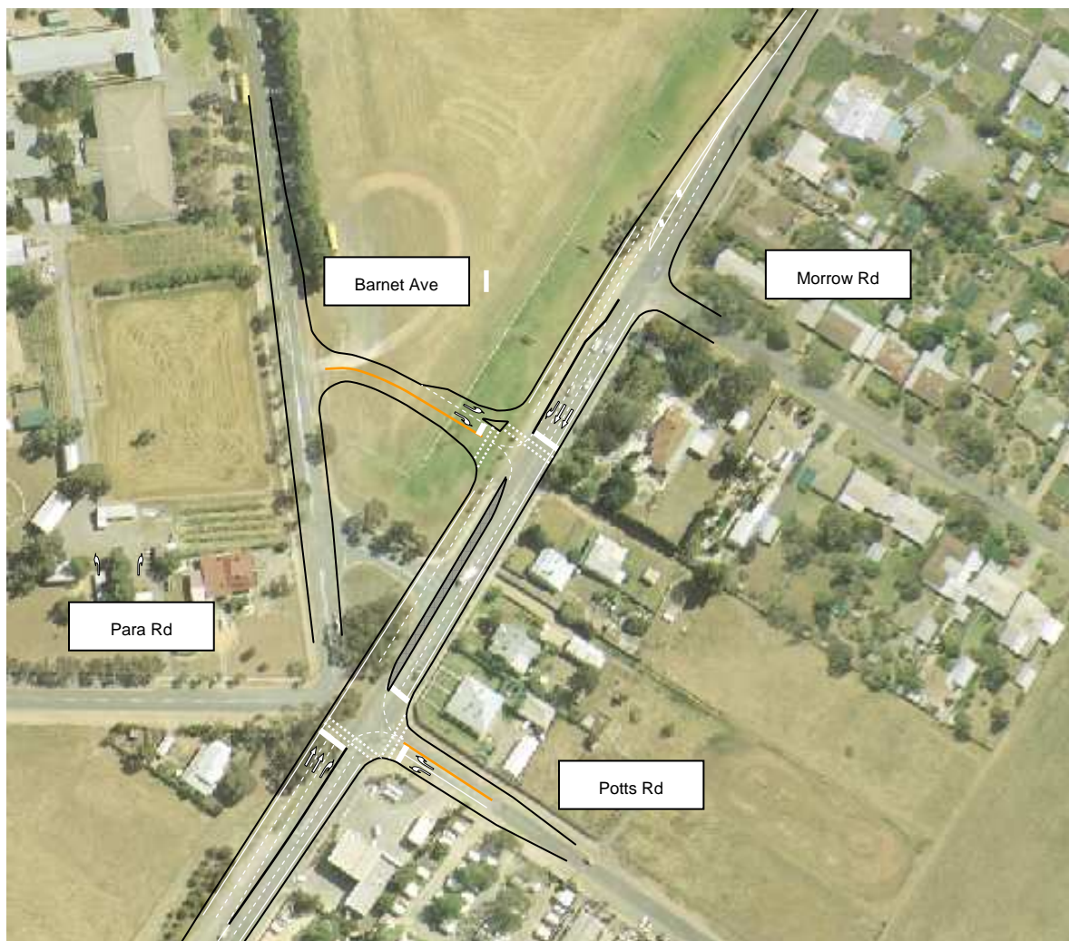
Figure 7-13 Concept traffic signals layout at Main North Road, Para Road and Potts Road
