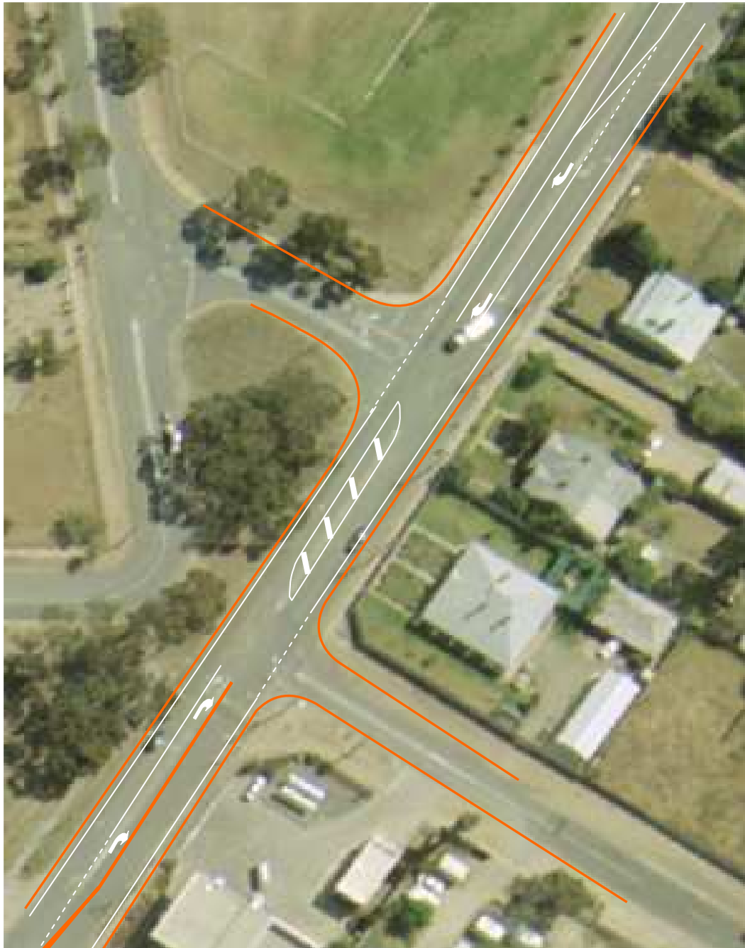
Figure 7-11 - Recommended short term treatment for Barnet St and Potts Road on Main North Road
