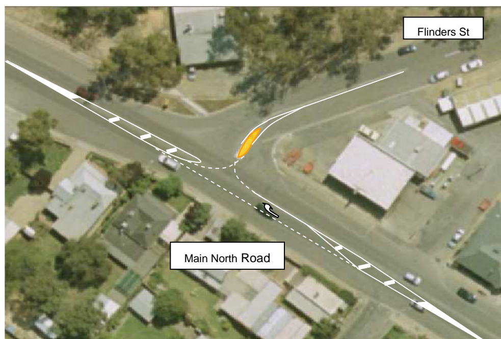
Figure 7-3 Concept of treatment at Main North Road and Flinders Street junction
